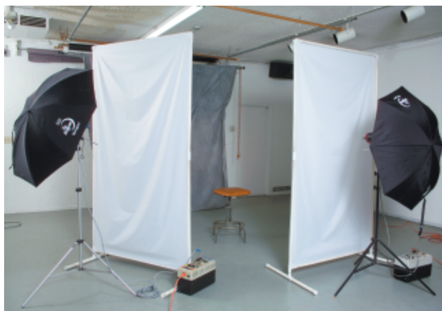
Figure 9. You can see the set-up for the soft-light shots here. The umbrella/light panel set-up is very effective at making soft light.
