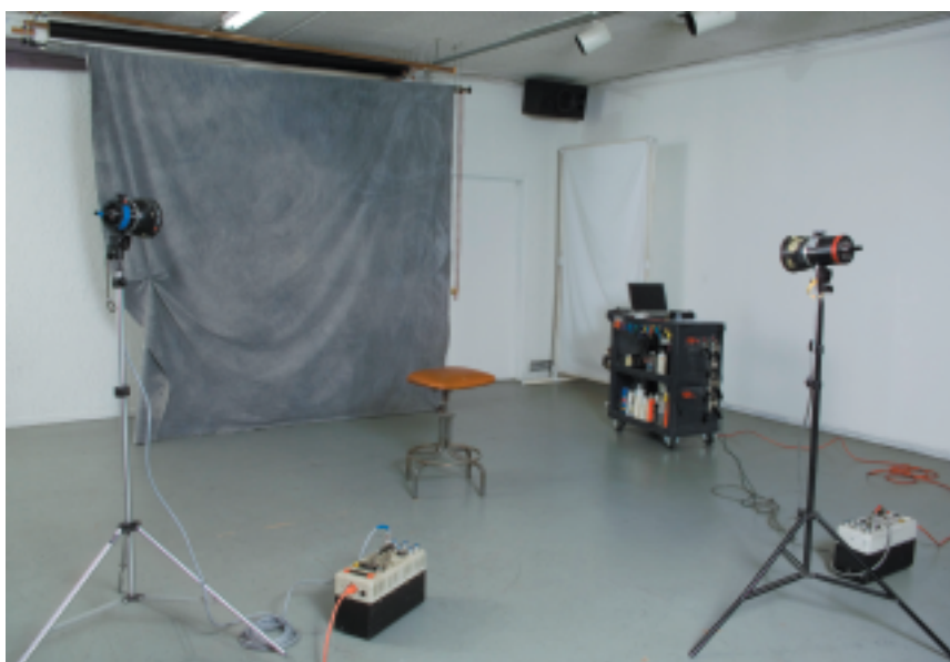
Figure 5. This shows the set-up for the hard light shots in my studio. Notice that I didn't use umbrellas or other tools to broaden the light source.
