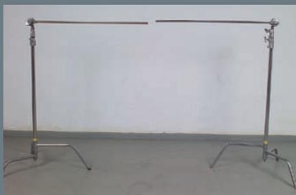
**Figure 4.** Two C-stands and a couple of extension arms can easily hold seamless paper or other background material.
