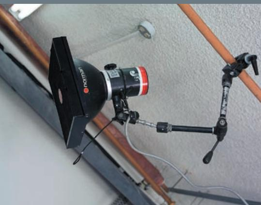
**Figure 3.** A Norman head mounted on a Bogen Magic Arm, which is mounted onto a super clamp.
