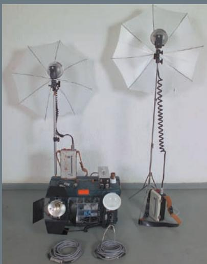
**Figure 9.** This entire battery-powered lighting system fits into one not-too-heavy case.
