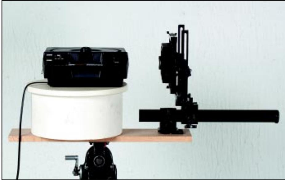
**Projector test:** The set-up for lens testing with a projector. A test slide is mounted in the projector and a diopter lens is mounted in the camera. This gives some information on sharpness, aberrations, and focus shift. I found it particularly useful in testing focus shift.
