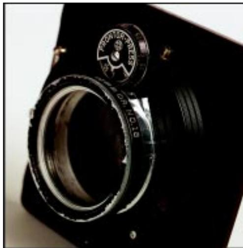
**Close-up of the shutter showing the adapter used to mount series 6 elements to the shutter.**
