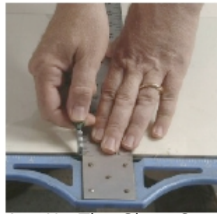
Lining Up The Glass Cutter With The T-Square © John Siskin All rights reserved
