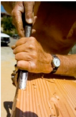
Gouging a Beam © John H. Siskin All rights reserved
