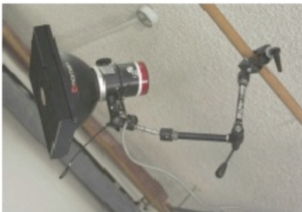
The Magic Arm is mounted into a super clamp. © John H. Siskin All rights reserved
