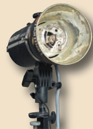
Figure 8. Reflector: really the simplest lighting tool; it gives direction to light.
