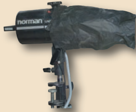
Figure 12. Cine foil is made of black aluminum foil that doesn't burn. It can be used in many ways to control light. This is wonderful stuff to have in the studio.
