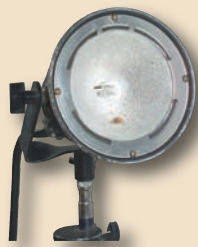
Figure 14. Spot. This is a tungsten light that throws a reasonably tight beam. Often these are adjustable, changing the size of the beam. Not as tight as an optical spot.
