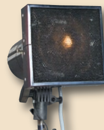
Figure 11. Grid or Honeycomb spot. This makes a very small spotlight that doesn't spread much. The grid is a honeycomb-shaped baffle that goes over the strobe. The small size of the individual holes keeps the light from becoming a larger spot.
