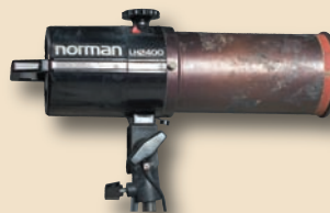
Figure 10. Snoots are very dramatic lights; they create a small pool or spot of light. Some manufacturers make more than one size snoot to give different sizes of spots. The size of the light from the snoot increases the further it is from the strobe.
