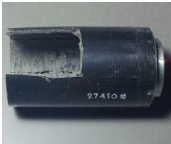
This is the tube made from PVC pipe. This is the heart of the device. You can see how the filter holder fits on the back.
