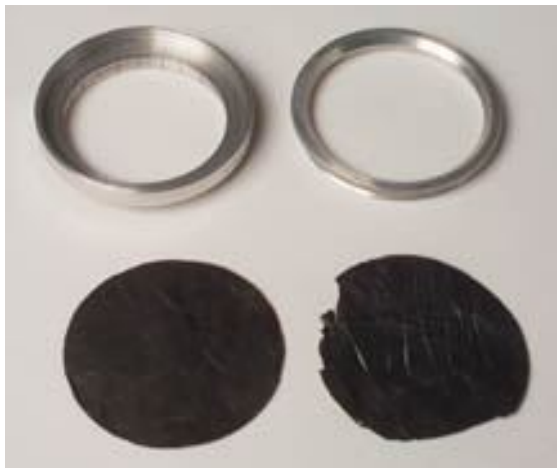
This is the filter holder and a couple of cookies. The one on the left hasn't been cut yet.
