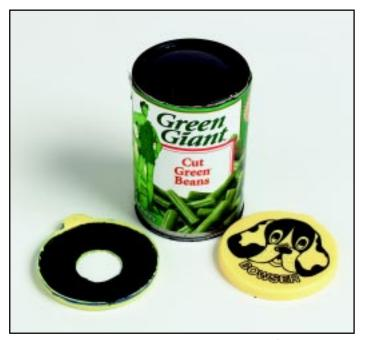
Can lens: Two +3 diopters are mounted in a can of Green Giant beans. The lenses are optical blanks available from the supply houses used by optometrists. Also shown is the lens cap and waterhouse stop-style aperture, made from dog food lids.
