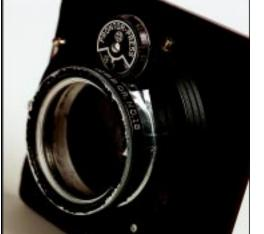
Close-up of the shutter showing the adapter used to mount series 6 elements to the shutter.
