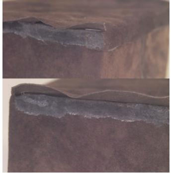
First cut the top right at the corner, not all the way to the edge of the box. Now, on the side where the seam is, wrap the tab onto the side you're working on and glue. Please note if you haven't coated these parts and waited for them to dry, you need to do that. You will also need to glue over the top of the tab. On the other side of the bellows, all that is
