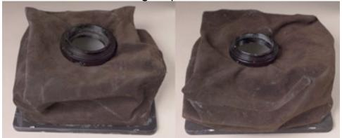
Check this on your camera. Position the hole in the bellows material between these pieces of the T-Mount and press them together. Secure them with the medium spring clamps from the outside of the lensboard.
