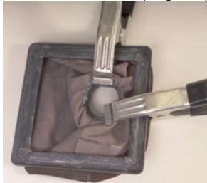
Reset the setscrews and allow drying for 12 hours. Your bellows is ready to go!
