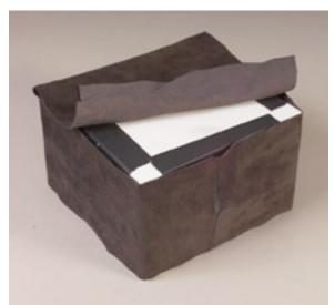
Next spread contact cement on the side of the bellows where the seam is, about 3/4 (.75) inches down. Spread cement on the inside of the top piece, remember these two pieces will meet, so make sure the cement will cover to the meeting place. A similar procedure will work for the sides. The key difference with gluing the sides is that cuts will need to be made to make the corners, and we'll need to do a little more gluing.
