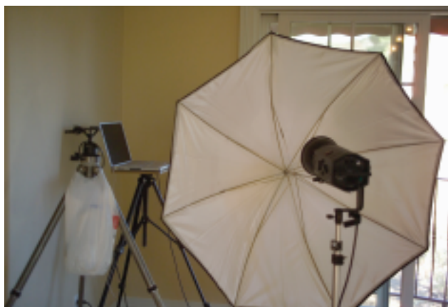
Figure 3. This shows the position of the largest strobe, the computer, and the camera. The strobe and the camera are close together to provide a similar angle for the light and the lens.
